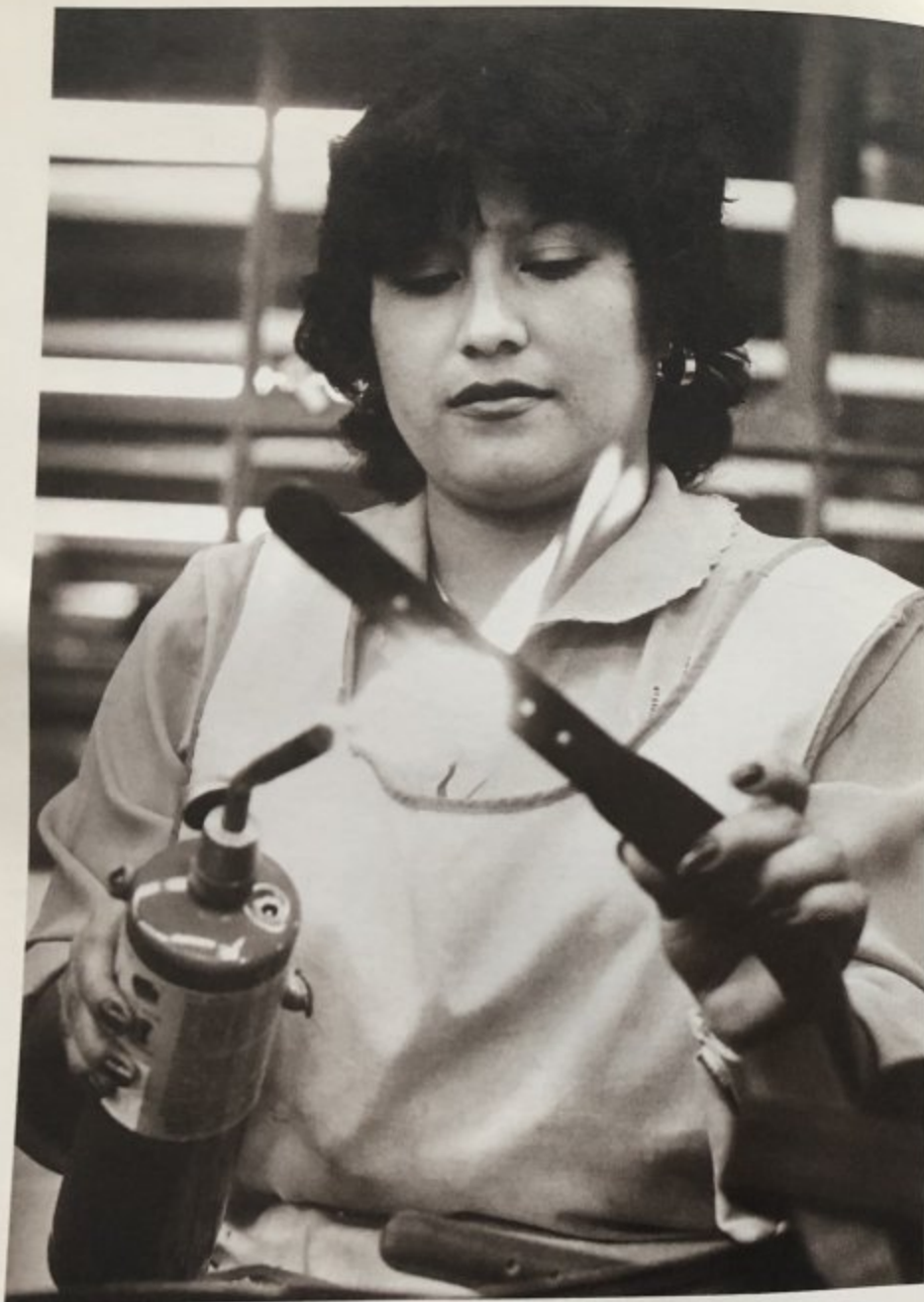
The Trimmer burns off loose threads with a live flame.
