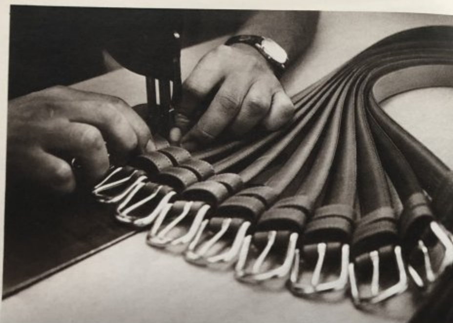
Every Coach® Belt has a solid brass buckle and two leather loops, carefully sewn on by a highly skilled sewing machine operator.
