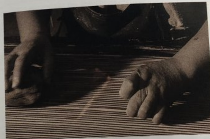
Belt straps are stacked across the table top. The edges are then buffed, stained, waxed and polished to the desired smoothness.
