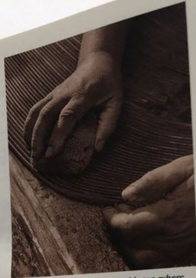
Belt straps are stacked across a table top where they are buffed, stained and waxed to the desired smoothness.
