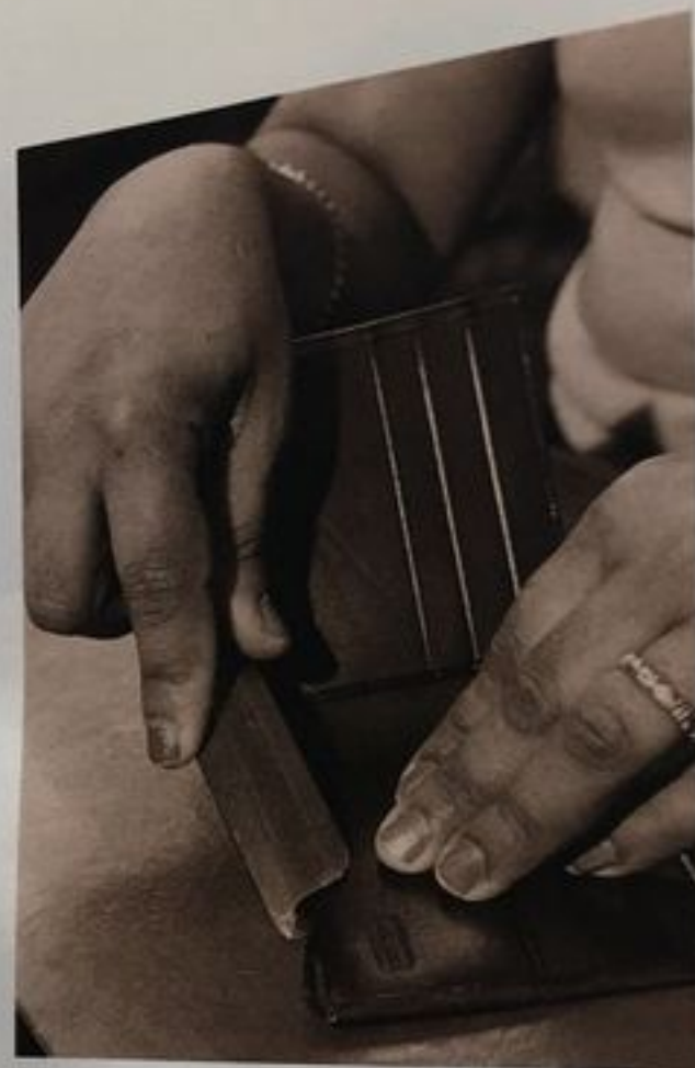
All of our wallets have hand-turned edges that are glued as well as sewn.
