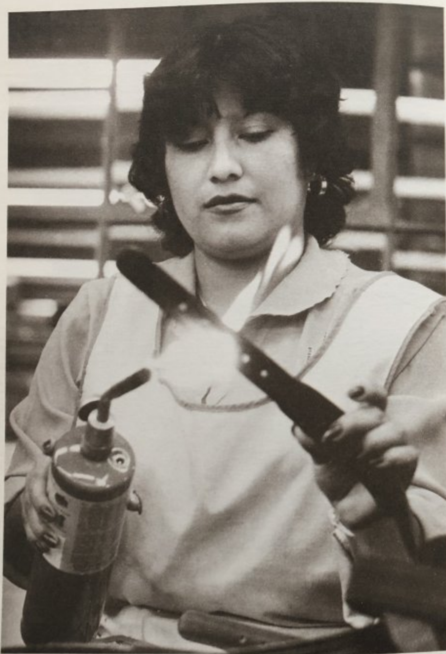
The Trimmer burns off loose threads with a live flame.
