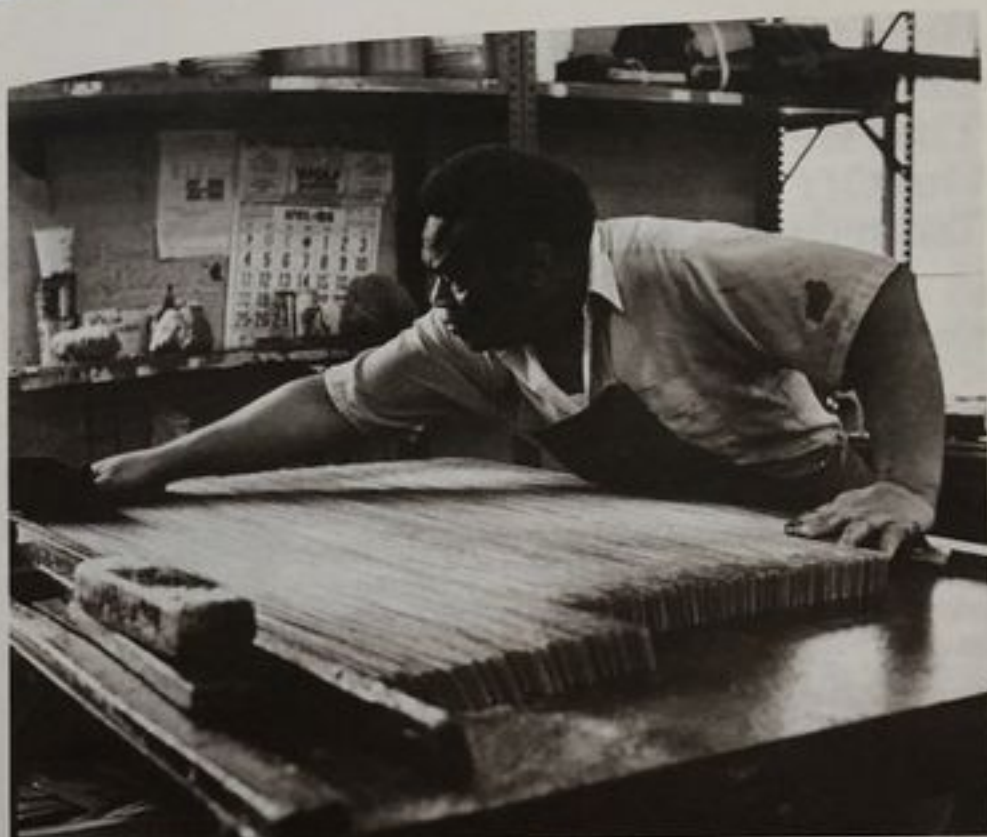
The Edge Finisher has stacked the belt straps across his table top where they are buffed, stained, and waxed to the desired smoothness.
