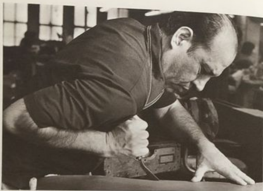
The Creaser applies a burnished edge to a leather strap with the help of a hot creasing iron and a little "elbow grease."
