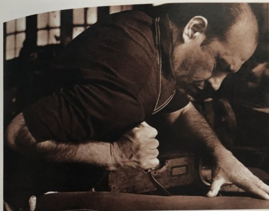
The Creaser applies a burnished edge to a leather strap with the help of a hot creasing iron and a little "elbow grease."
