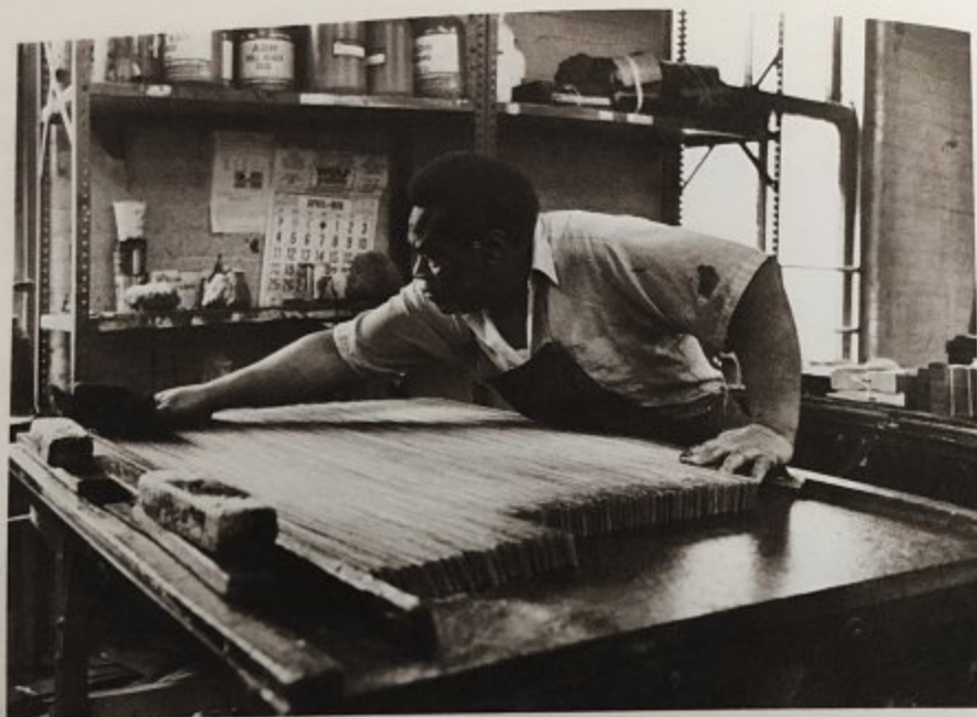
The Edge Finisher has stacked the belt straps across his table top where they are buffed, stained, and waxed to the desired smoothness.
