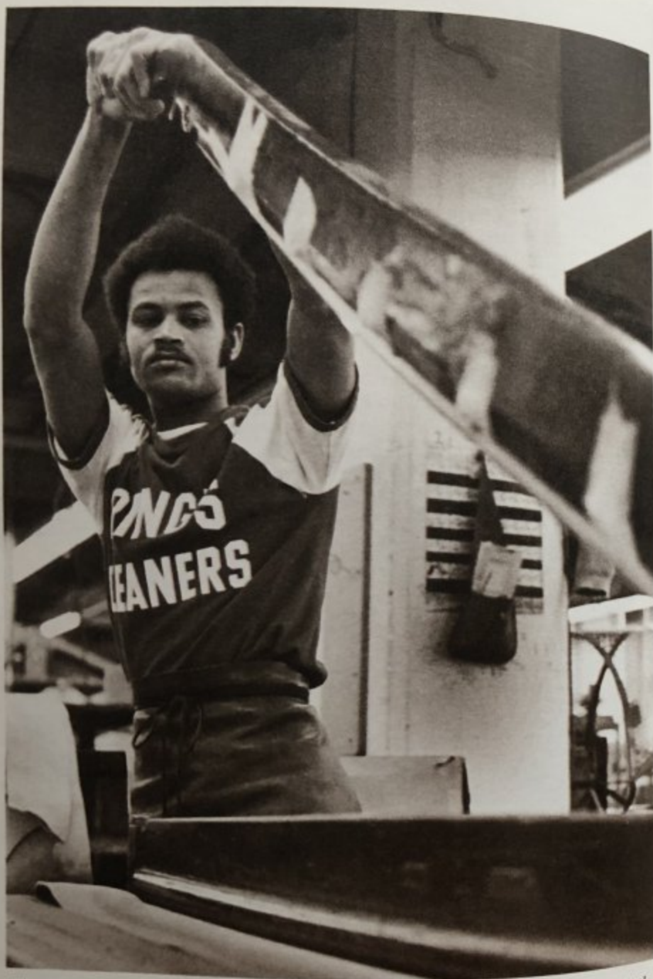
The Shear Cutter trims the hide and cuts it into rough blocks with this fifty-four inch steel blade. The leather blocks will then be slit down to accurate belt widths.
